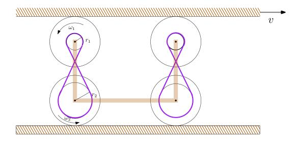
The cart represented in the figure has been assembled by connecting together four identical cylinders, with mass m and radius R, using a rigid structure with negligible mass. The cylinders rotate without slipping on the horizontal planes they are in contact with.
